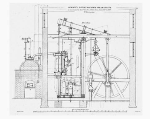
Fig. 5: The caption for this technical drawing reads "Mr. Watt's Patent Rotative Steam Engine as constructed by Messrs. Boulton & Watt, Soho, from 1787 to 1800. 10 Horse power." By 1787, the engine had evolved considerably from the earlier versions, using the sun-and-planet gear to drive the large wheel; the Watt linkage to connect the beam with the cylinder, on the left; and even Watt's feedbackdriven flyball governor—the two balls hanging
